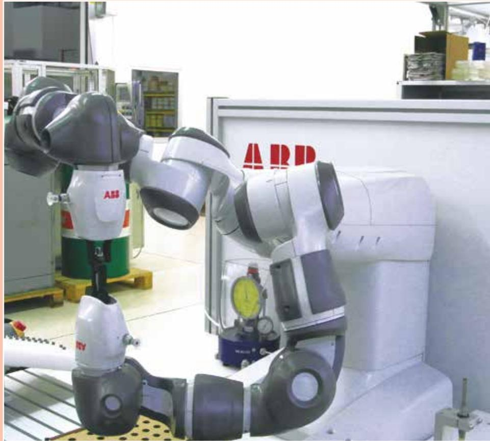
second component from the corresponding tray; then, the valve, which has already been tested, is assembled, as the robot is capable to move in space moving back to the same spot with an accuracy of 0.02 mm.
